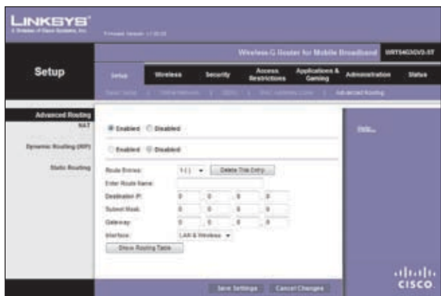
Setup > Advanced Routing
